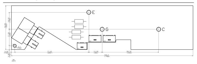
Maximum driver height: 13mm measured from the bottom layer
