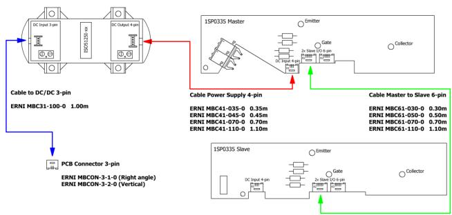
Fig. 11 Cable arrangement for 1SP0335 (Master only or Master and Slave) and DC-DC converter ISO5125I All cables are delivered with straight plugs on both sides.
