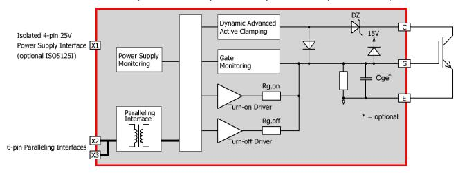
Fig. 3 Basic schematic of the 1SP0335D drivers
