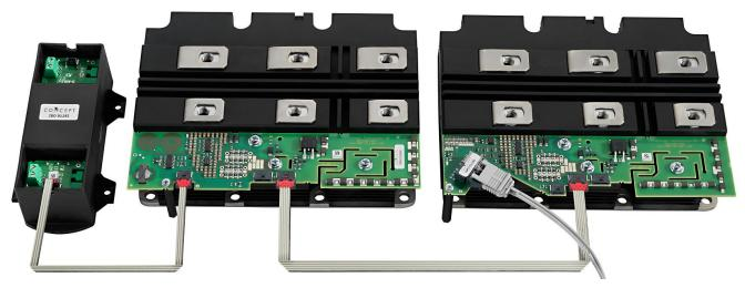
Fig. 1 1SP0335D (slave) with 1SP0335V (master) each screwed onto a 6.5kV IGBT module (left: DC/DC converter ISO5125I connected to 1SP0335D)
