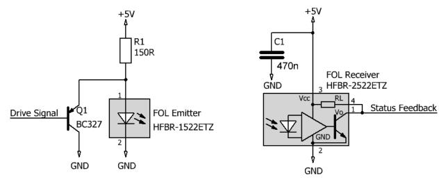
Fig. 17 Recommended circuitry for the "versatile" fiber-optic links (1SP0335V)
