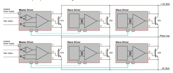
Fig. 4 Principle of parallel connection of 1SP0335 drivers with one master and two slaves in a half-bridge configuration (example)
