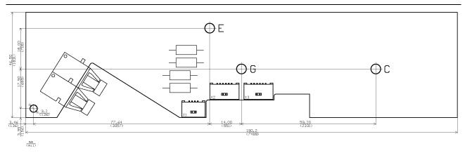
Maximum driver height: 10mm measured from the bottom layer
