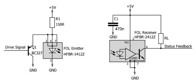
Fig. 18 Recommended circuitry for the "ST" fiber-optic links (1SP0335S)
