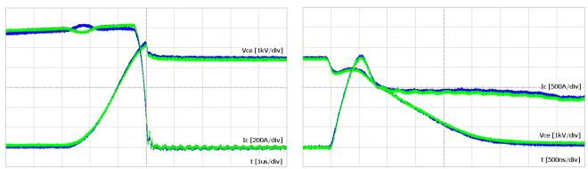
Fig. 21 Turn-off (left) and turn-on (right) behavior of two 600A/6500V IGBT modules in parallel connection at a DC-link voltage of 4450V and a collector current of 1200A each
