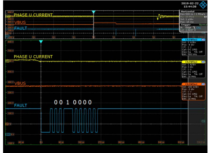
Figure 19. Inverter Shutdown After a Line Overvoltage Condition.
