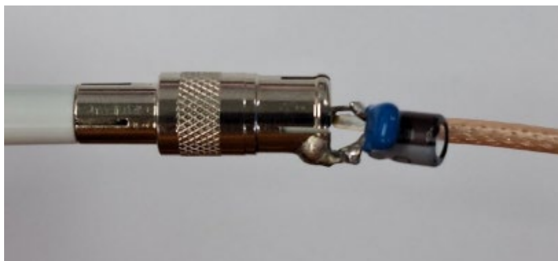
Figure 28 – Oscilloscope Probe with Probe Master ( www.probemaster.com ) 4987A BNC Adapter. (Modified with wires for ripple measurement, and two parallel decoupling capacitors added)
