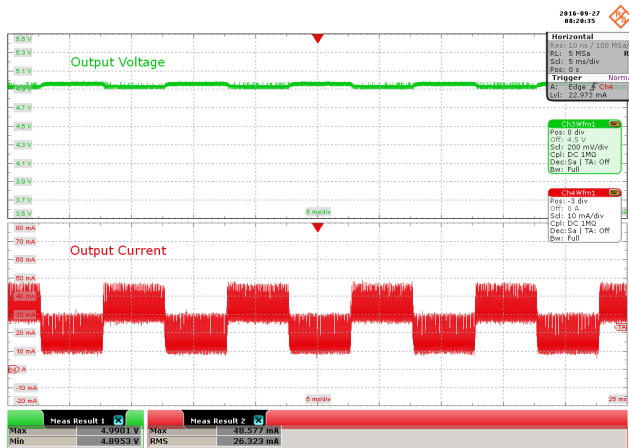
Figure 22 – 85 VAC Input. V_{OUT} , 200 mV / div. I_{OUT} , 10 mA / div., 5 ms / div. V_{MAX} : 4.9901 V. V_{MIN} : 4.8953 V.
