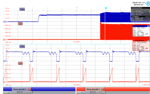
Figure 38 – 265 VAC, 50 Hz. Upper: V_{DRAIN} , 200 V / div., 20 ms / div. Lower: I_{DRAIN} , 200 mA / div., 20 ms / div. Zoom: 10 \mu s / div. Measured V_{PK} = 519 V_{PK} . Measured I_{PK} = 950 mA_{PK} .
