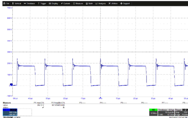
Figure 28 – Input (Min.): 85 VAC, Load: 2 A CH1, V_{DS} , 100 V / div., 10 \mu s / div. V_{DS} (Max.): 242 V. Derating: 33.38 %.
