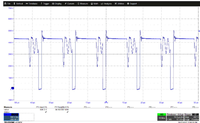
Figure 29 – Input (Max.): 265 VAC, Load: 2 A CH1, V_{DS} , 100 V / div., 10 \mu s / div. V_{DS} (Max.): 504.5 V. Derating: 69.59 %.
