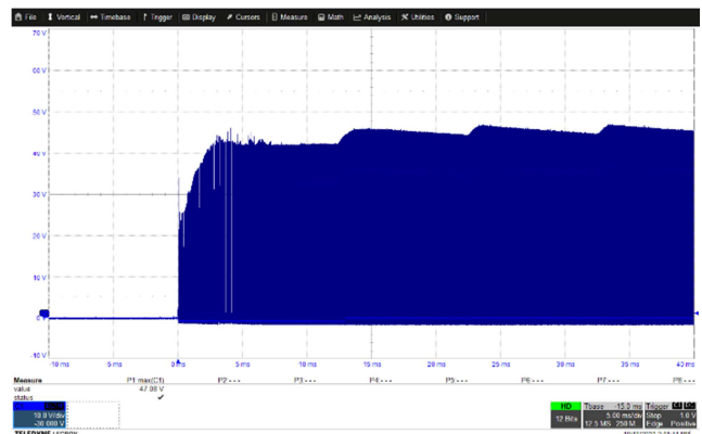
Figure 37 – Input (Max.): 265 VAC, Load: 2 A. CH1, V_{DS} , 10 V / div., 5 ms / div. V_{DS} (Max.): 47.08 V. Derating: 78.47 %.
