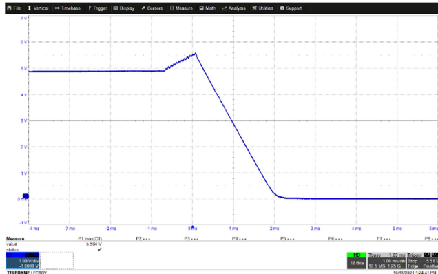
Figure 40 – Input (Min.): 85 VAC, Load: 2 A. CH1, V_{OUT} , 1 V / div., 1 ms / div. V_{OUT} (Max.): 5.584 V.
