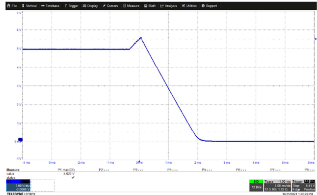
Figure 41 – Input (Max.): 265 VAC, Load: 2 A. CH1, V_{OUT} , 1 V / div., 1 ms / div. V_{OUT} (Max.): 5.622 V.
