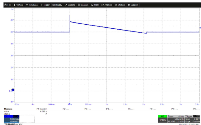
Figure 43 – Input (Max.): 265 VAC, Load: 0 A. CH1, V_{OUT} , 1 V / div., 500 ms / div. V_{OUT} (Max.): 6.398 V.
