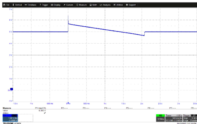
Figure 42 – Input (Min.): 85 VAC, Load: 0 A. CH1, V_{OUT} , 1 V / div., 500 ms / div. V_{OUT} (Max.): 6.356 V.
