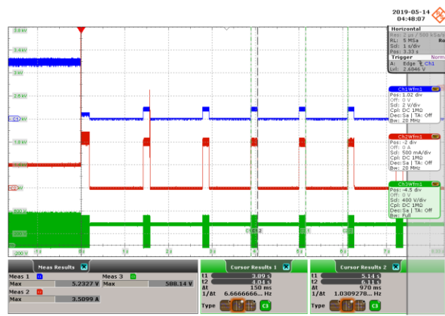
Figure 73 – 265 VAC, Normal Operation. CH1: V_{OUT} , 2 V / div., 1 s / div. CH2: I_{OUT} , 500 mA / div., 1 s / div. CH3: V_{DS} , 400 V / div., 1 s / div. t_{AR(ON)} : 150 ms. t_{AR(OFF)} : 0.97 s.
