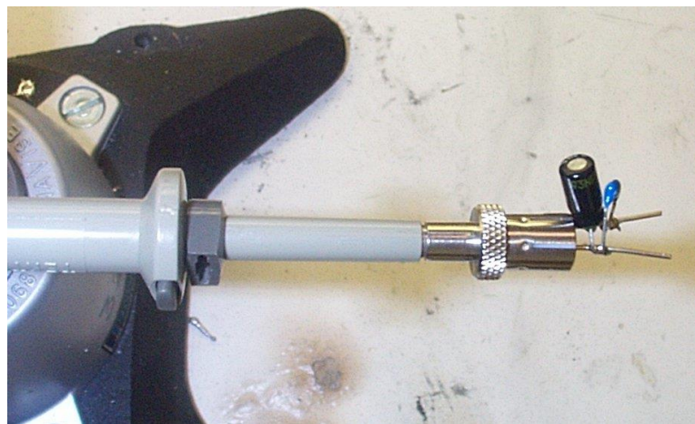
Figure 77 – Oscilloscope Probe with Probe Master ( www.probemaster.com ) 4987A BNC Adapter. (Modified with wires for ripple measurement, and two parallel decoupling capacitors added)
