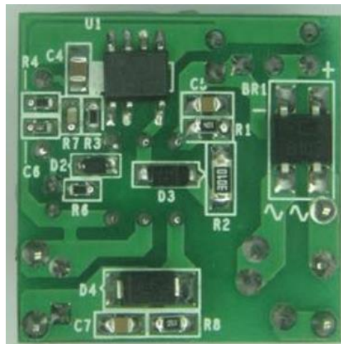
Figure 2 – Populated Circuit Board Photograph, Bottom.
