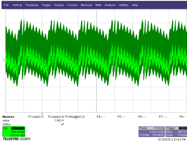
Figure 49 – Output Ripple. 90 VAC, 2 A Load 5 ms / 200 m V / div.
