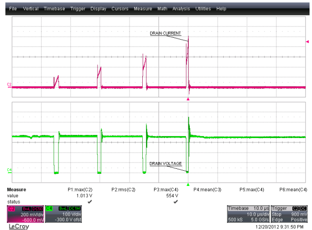
Figure 40 – 265 VAC, 50 Hz Start-up. Upper: I_{DRAIN} , 200 mA / div. Lower: V_{DRAIN} , 100 V, 10 \mu s / div.
