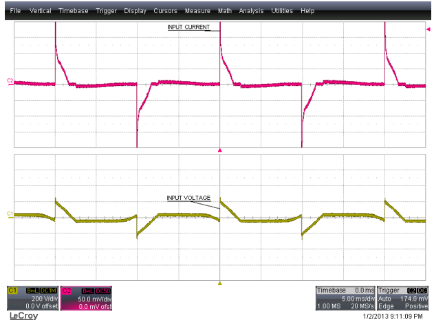
Figure 60 – 45° Conduction Angle. Upper: I_{IN} , 50 mA / div. Lower: V_{IN} , 200 V, 5 ms / div.
