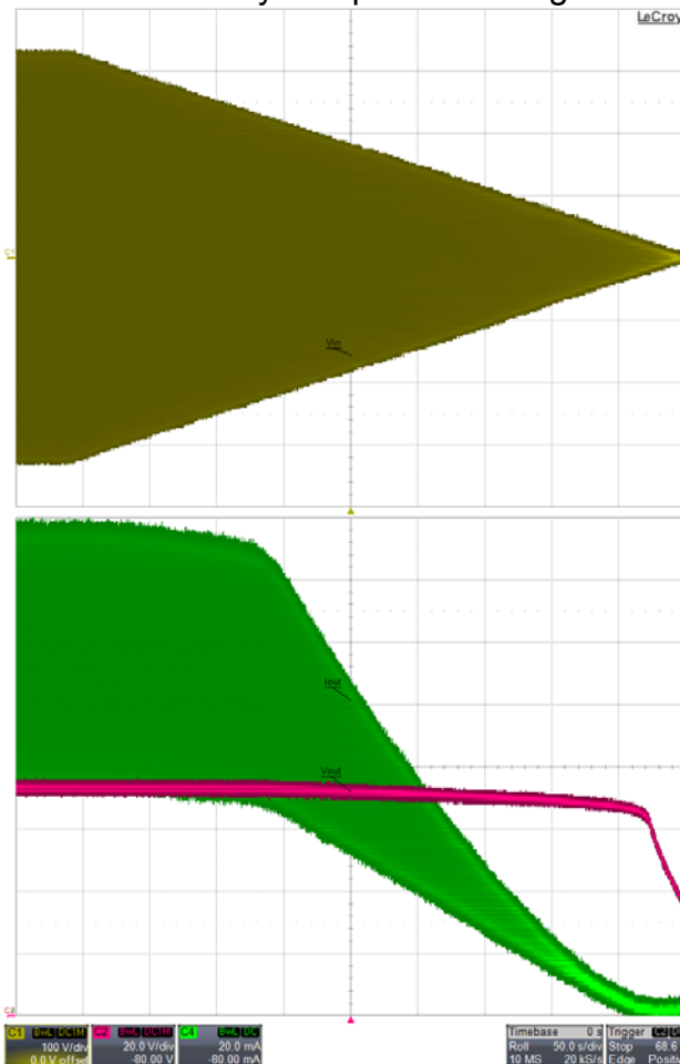
Figure 47 – Brown-out Test at 0.5 V / s. The Unit is Able to Operate Normally Without Any Failure and Without Flicker. 230 V-0-230 V Ch1: V_{IN} ; 100 V / div. Ch2: V_{OUT} ; 20 V / div. Ch3: I_{OUT} ; 20 mA / div. Time Scale: 50 s / div.
