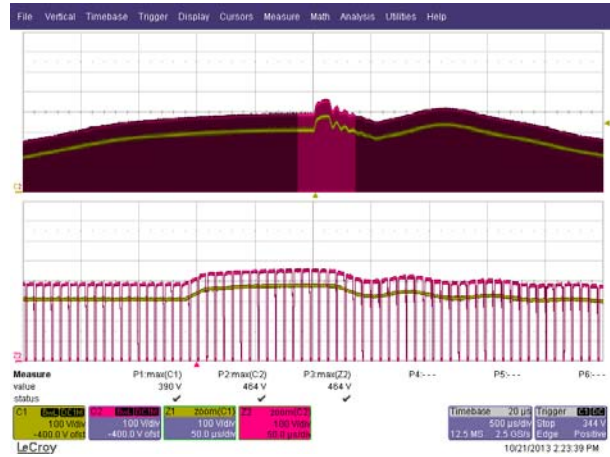
Figure 218 – Differential Line Surge at 500 V / 90°. Peak Drain Voltage Recorded is 464 V. Ch1: V BULK ; 100 V / div. F1: V DRAIN ; 200 V / div. Time Scale: 500 μs / div. Zoom time Scale: 50 μs / div.
