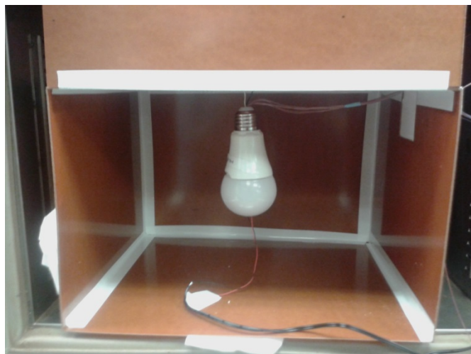
Figure 18 – Thermal Unit Thermocouple Measurement Set-up.
