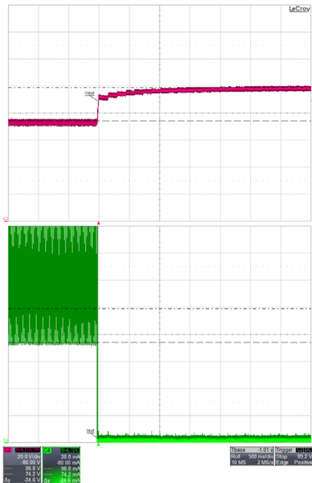
Figure 44 – No-load Protection when Load is Disconnected. 265 V / 50 Hz. Ch2: V OUT ; 20 V / div. Ch3: I OUT ; 50 mA / div. Time Scale: 500 ms / div.
