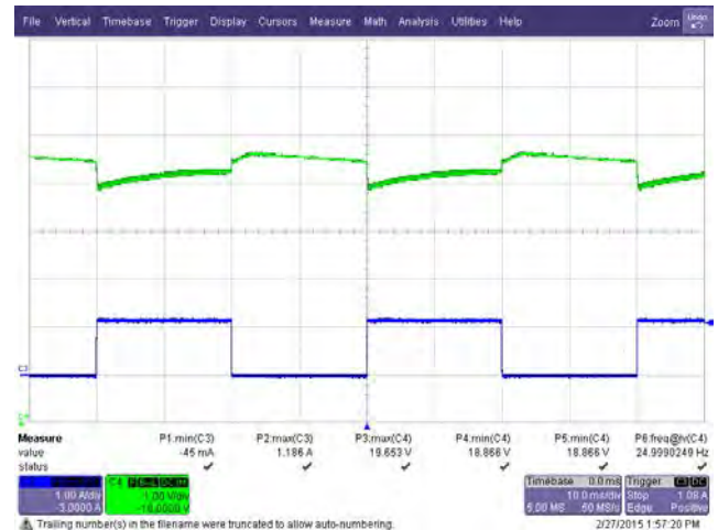
Figure 26 – Transient Response, 115 VAC, 0% <--> 50% Step Load. Upper: V OUT , 2.0 V / div. Lower: I OUT , 1 A / div., 10 ms / div.
