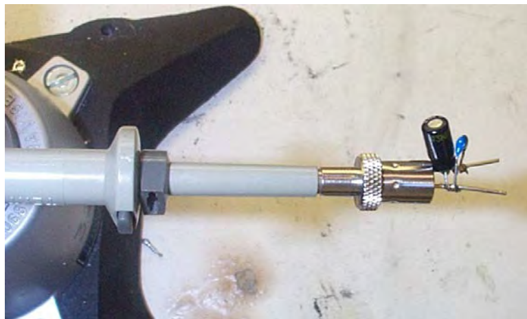
Figure 37 – Oscilloscope Probe with Probe Master 5125BA BNC Adapter (Modified with Wires for Probe Ground for Ripple Measurement, and Two Parallel Decoupling Capacitors Added).
