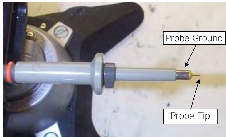
Figure 13 – Oscilloscope Probe Prepared for Ripple Measurement. (End Cap and Ground Lead Removed)
