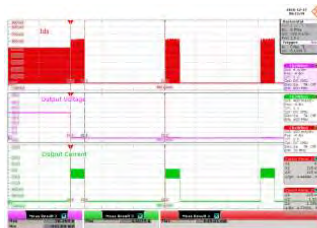
Figure 39 – 265 VAC Input. Condition: 20 V – Shorted. Auto-Restart: 1.51 s. Upper: I_{DS} , 100 mA / div. Middle: V_{OUT} , 4 V / div. Lower: I_{OUT} , 400 mA / div., 500 ms / div.
