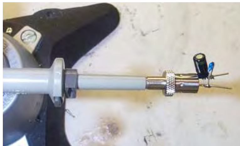
Figure 14 – Oscilloscope Probe with Probe Master ( www.probemaster.com ) 4987A BNC Adapter. (Modified with wires for ripple measurement, and two parallel decoupling capacitors added)
