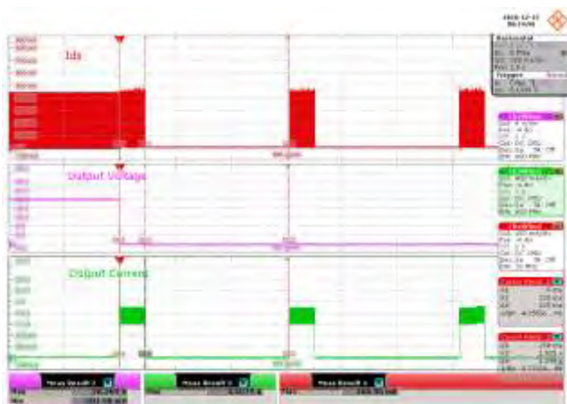
Figure 38 – 85 VAC Input. Condition: 20 V – Shorted. Auto-Restart: 1.525 s. Upper: I_{DS} , 100 mA / div. Middle: V_{OUT} , 4 V / div. Lower: I_{OUT} , 400 mA / div., 500 ms / div.
