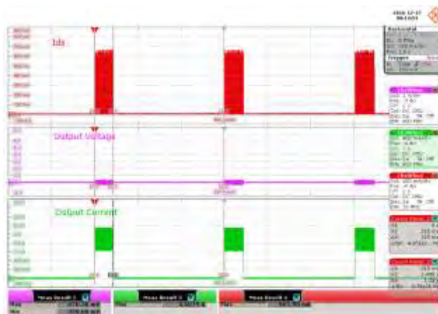
Figure 37 – 265 VAC Input. Condition: 20 V – Shorted. Auto-Restart: 1.495 s. Upper: I_{DS} , 100 mA / div. Middle: V_{OUT} , 1 V / div. Lower: I_{OUT} , 400 mA / div., 500 ms / div.
