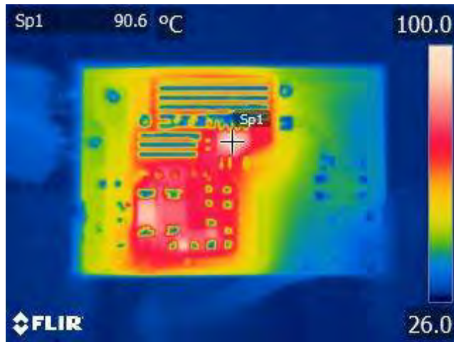
U1 – LinkSwitch-CV. Spot Temperature – 90.6 °C.
